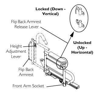
FIGURE 7.2 Adjusting Flip Back Armrests
